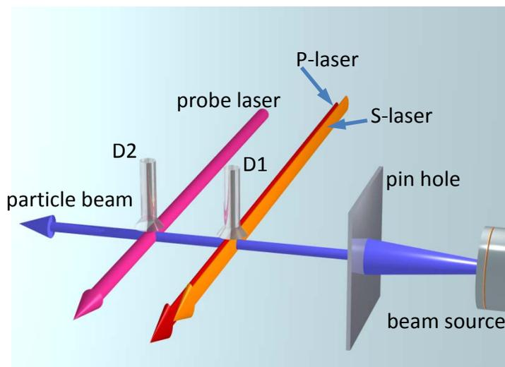
**Figure 3:** A typical setup for the implementation of STIRAP with continuous lasers and an atomic or molecular beam. The transfer occurs in the region where the S- and P-laser beams overlap. The detector D1 monitors fluorescence, if any, emitted from state 2 in that region. Detector 2 monitors the population of state 3 by laser-induced fluorescence.
